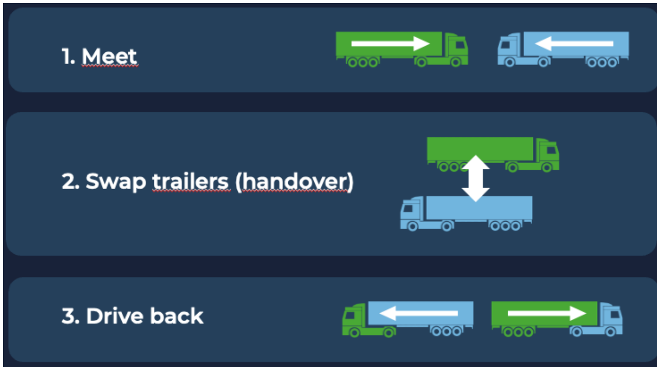
Figure 2: Relay transport is based on swapping trailers or containers along routes
