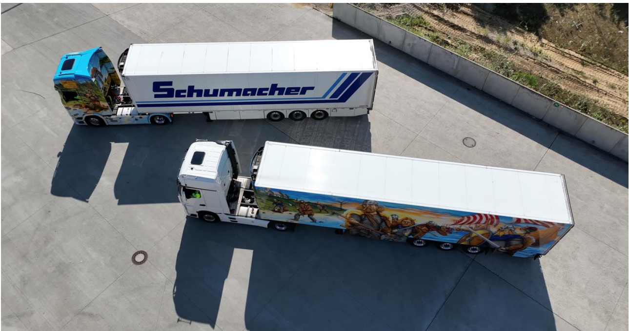
Figure 3: Two trucks swapping trailers. Any empty parking space can serve as a handover station.
